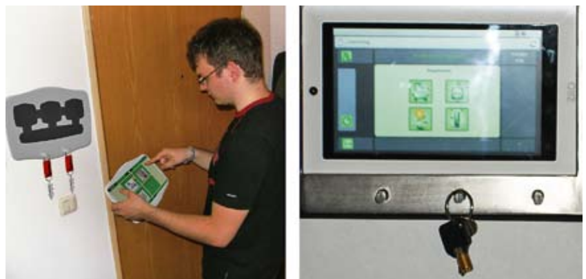
Fig. 4: Left: paper mock-up of a Smart Living key-holder panel. Right: actually built prototype using a ZIIO tablet computer as display unit. The key hooks serve as electrical contacts, too.
