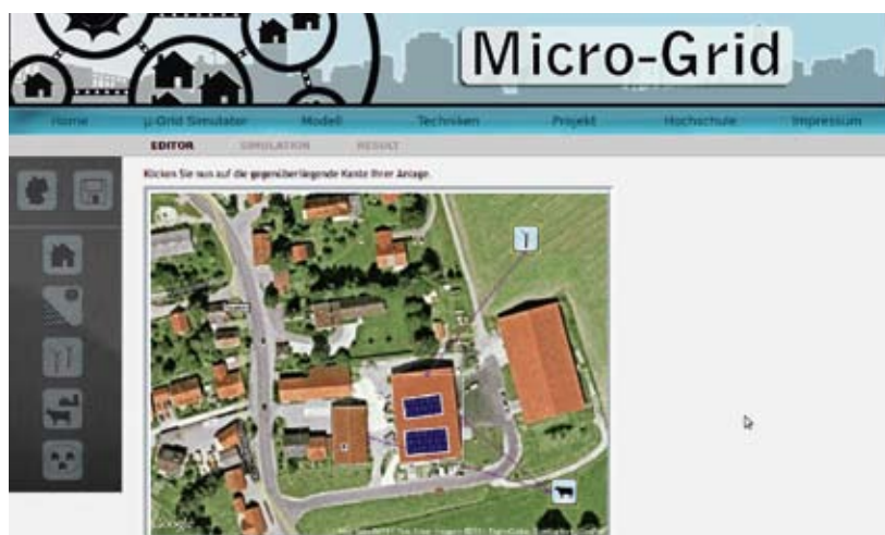
Fig. 7: Screenshot of the Micro-Grid Simulator. Via a web-interface a user can place renewable energy generators (solar panels and wind turbines) on a section of a Google map and then have the simulator perform a cost-benefit analysis on the basis of recorded regional weather data sets.
