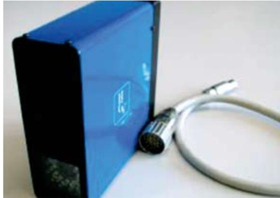
Figure 6. 3D-robot sensor [6]
