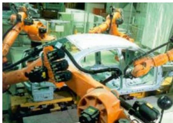
Figure 2. In-line-gauging station with gauging robots [1]
