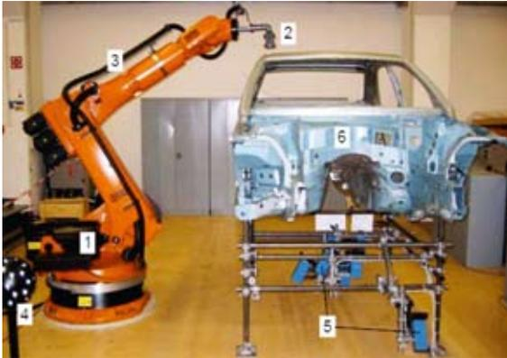
Figure 5. Test set-up with KUKA/HGV inline-measuring system
