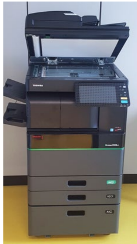
The positive experiences in the pilot project were convincing: The Faculty of Business is using a further environmental copier manufactured by Toshiba. The special feature is the blue toner. When the printed paper is no longer needed, the toner can be neutralised using a second device and the paper can be reused.
