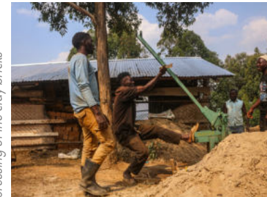
Pressen der Ziegelsteine pressing of the clay bricks
