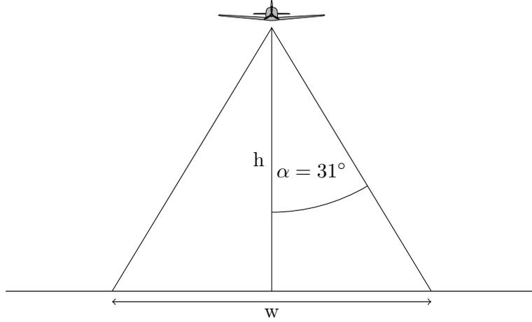
Figure 2: Raspberry Pi Camera V2.1 pointing down - width  $w$  at ground
