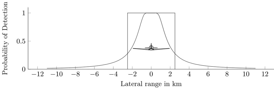
Figure 9: Definite Range and Inverse Cube Sensors with equal sweep width  $W = 5$  km
