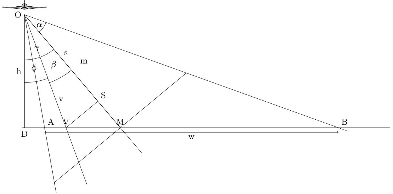
Figure 3: Raspberry Pi Camera V2.1 looking 40 degrees to the side
