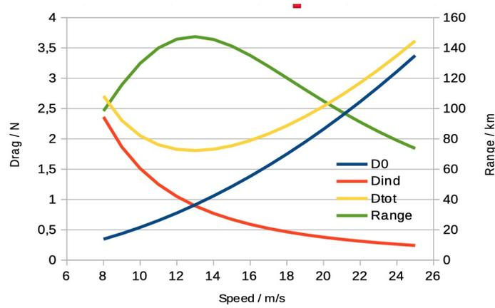
Figure 12: Drag and Range vs. speed
