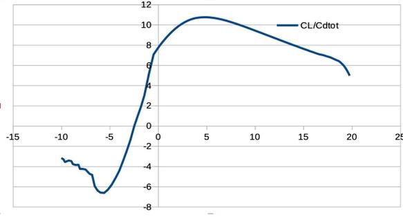
Figure 8:  $C_L/C_D$  vs. angle of attack
