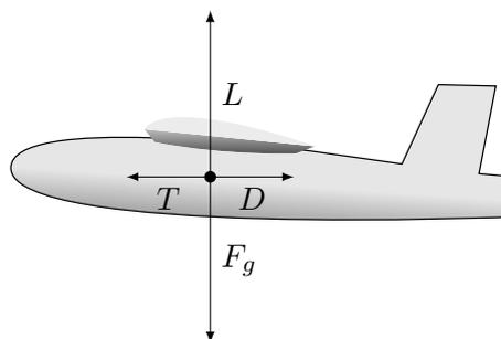
Figure 1: Condition for level flight - weight force equals lift and drag is equal thrust
