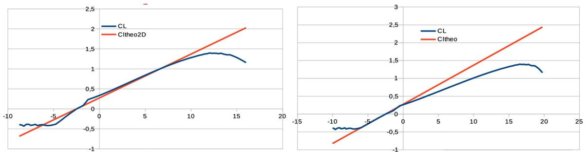
Figure 7: Lift of the infinite wing (left) vs. lift of the finite wing with aspect ratio of 5.63 (right)
