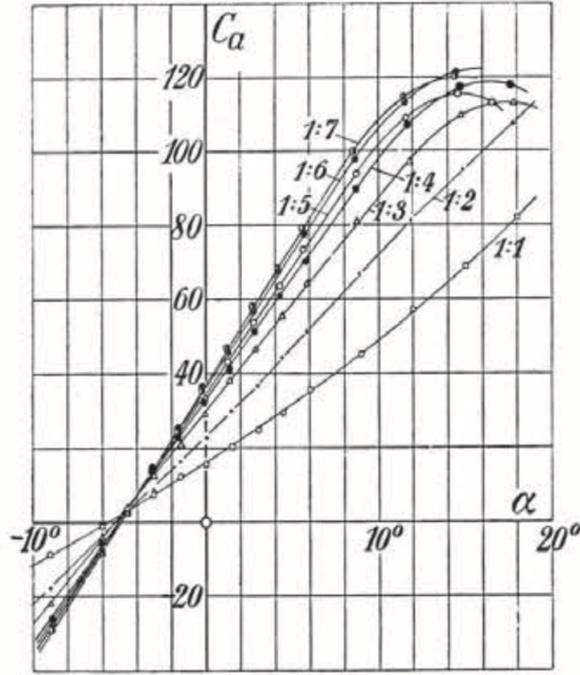
Figure 4:  $C_a (= C_l)$  vs. angle of attack for different wing aspect ratios from [3, p.51]
