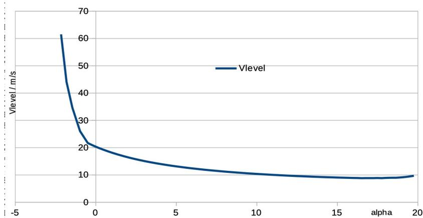
Figure 9: Velocity V for level flight vs. angle of attack
