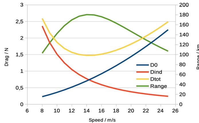
Figure 13: Drag and Range vs. speed for  $C_{D0} = 0.02$
