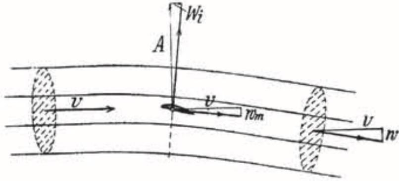
Figure 6: Airflow showing the induced angle  $\alpha_i$  due to induced drag  $W_i$  (from [3][p. 37])
