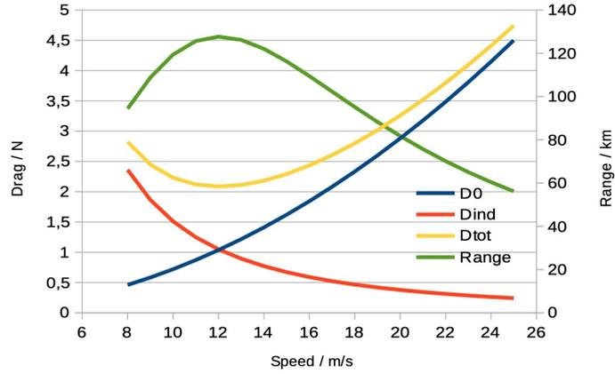
Figure 14: Drag and Range vs. speed for  $C_{D0} = 0.04$
