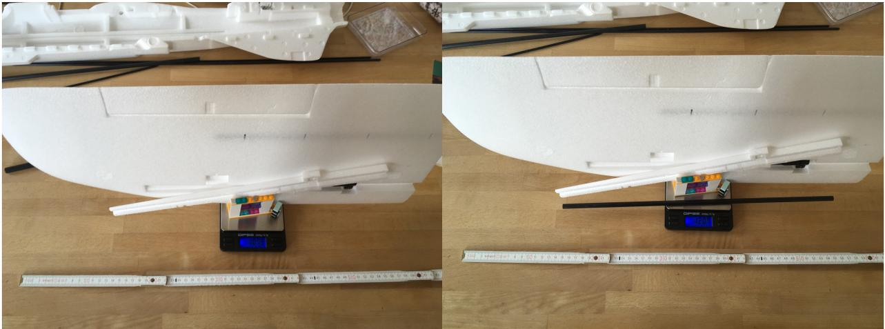
Figure 7: Left wing foam only 107.9g and with fiber beam 120.7g
