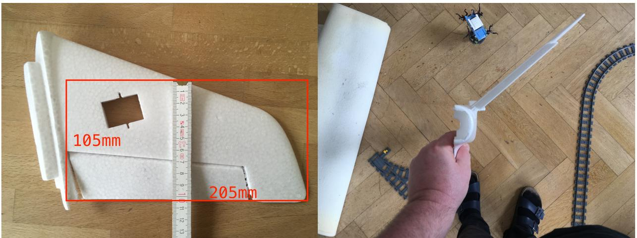
Figure 14: vtail area sketch and vtail angle (right)
