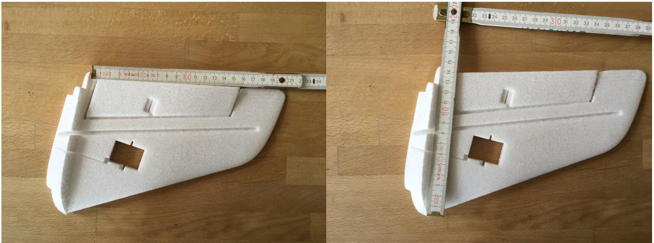
Figure 13: The vtail span is 205mm and has a width of 140mm at the base
