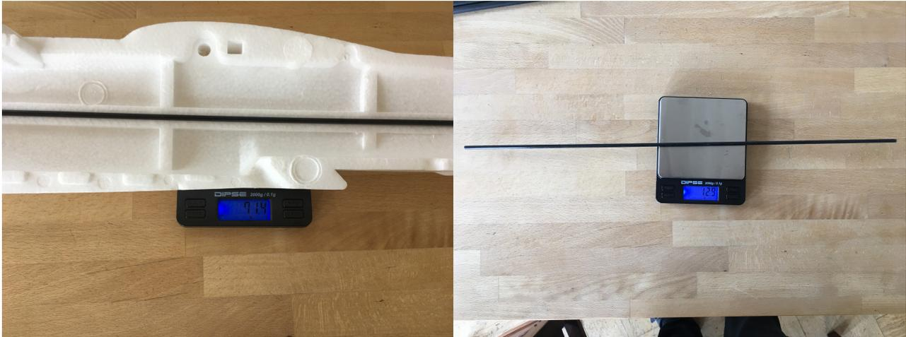
Figure 2: Fuselage half foam and fiber beam 71.4g and fiber beam only with 12.9g
