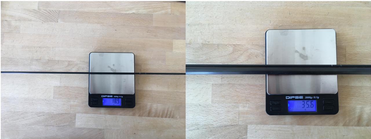
Figure 9: left: wing fuselage rear beam (18.9g) , right: wing fuselage rear and front beam (35.6g)
