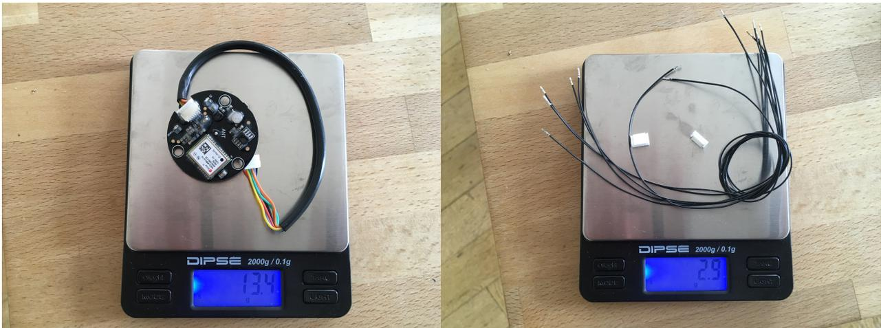
Figure 19: GPS (13.4g) and JST-GH 6 wire 12 inch cable (2.9g)
