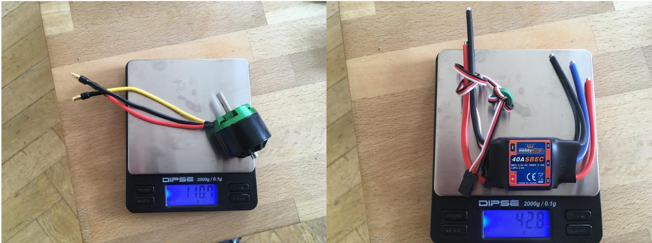
Figure 24: Left: Cobra 2814/20 850kV motor (110.7g), Right: Hobbyking 40A ESC (42.8g)
