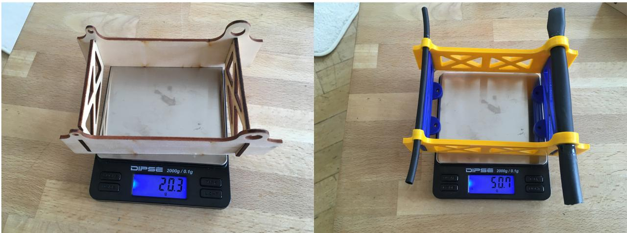
Figure 5: Fuselage reinforcement box. Left: Original wood version (20.3g). Right: 3D Print version (50.7g)
