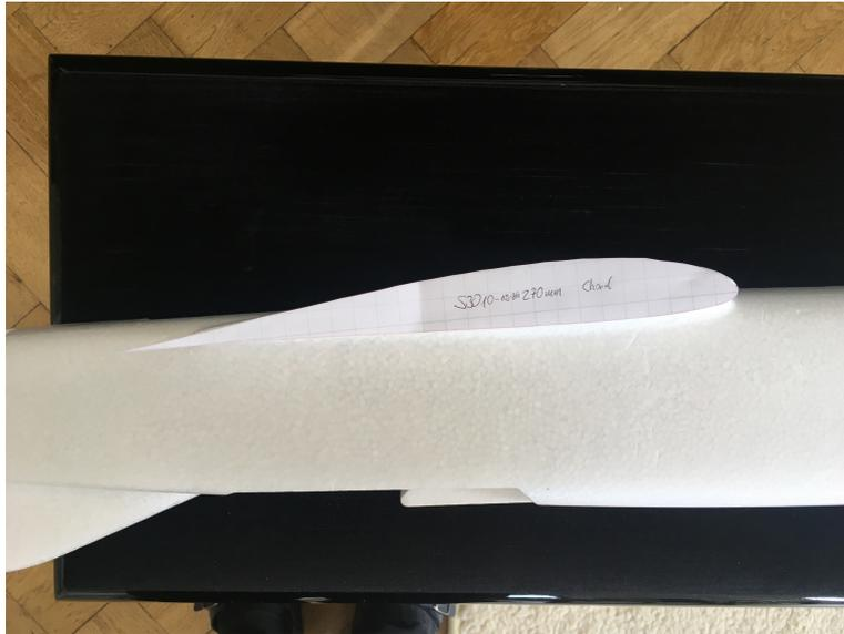
Figure 11: Wing airfoil shape S3010 with chord length of 270mm
