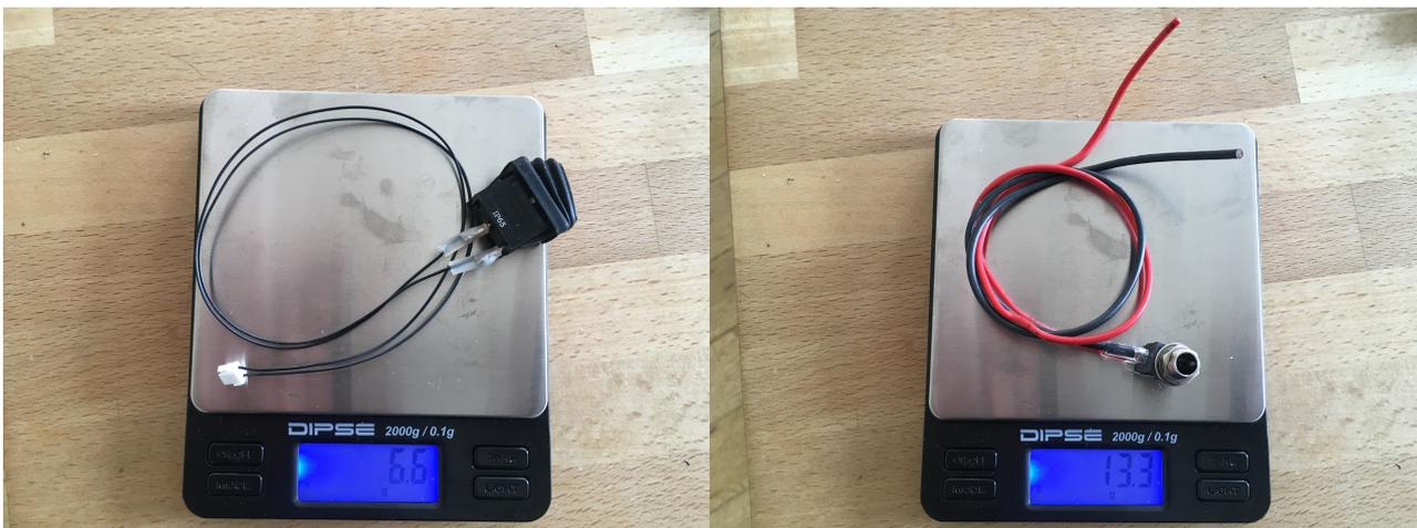
Figure 22: Left: power switch (6.6g), Right: charge connector (13.3g)
