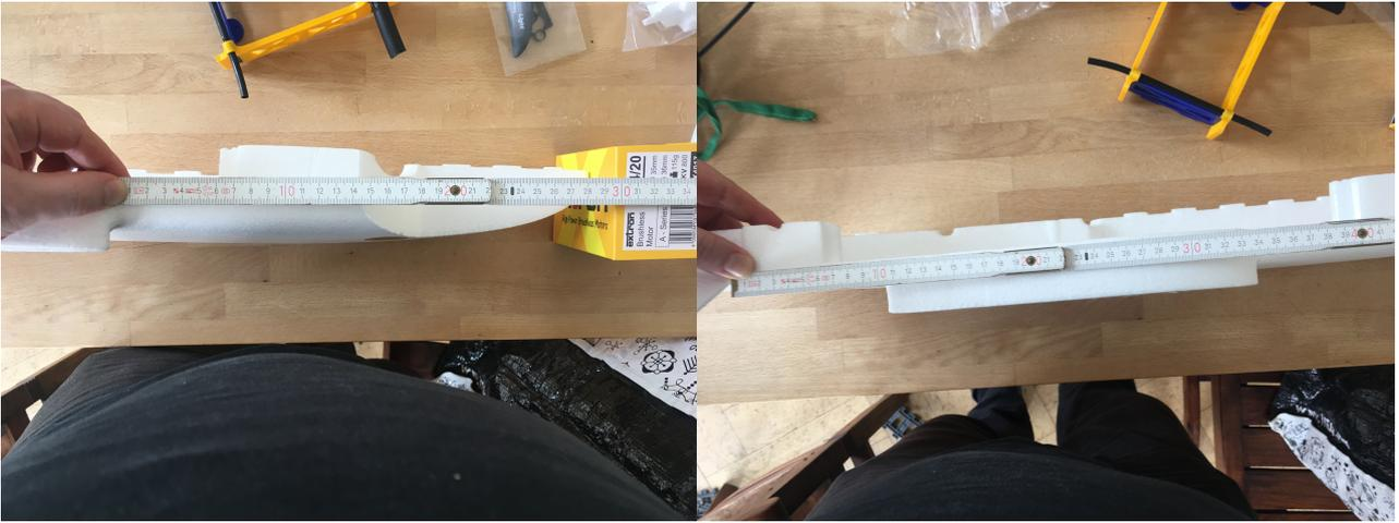
Figure 15: Left: fuselage nose to main wing leading edge 300mm. Right: Main wing leading edge to vtail leading edge 340mm
