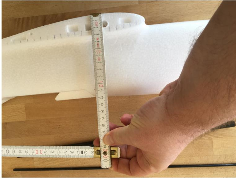
Figure 4: Fuselage height of 120mm
