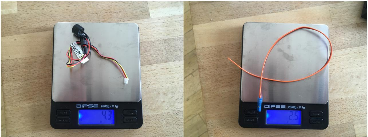
Figure 20: Beeper cable (4.3g) and 30cm servo cable ( $0.14 \text{ mm}^2$ ) (2.5g)
