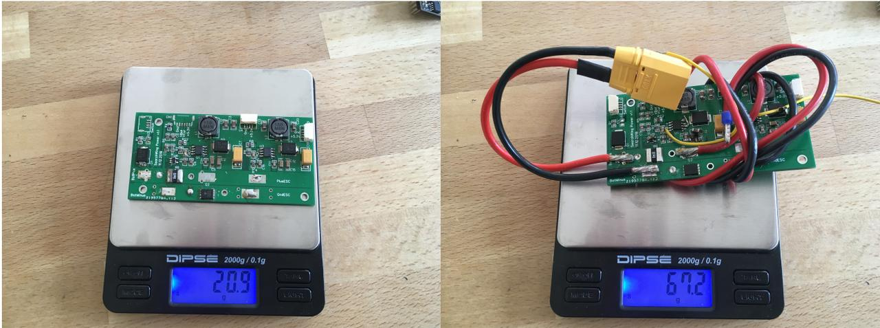
Figure 21: Left: Power module (20.9g), Right: Power module with cable and XT90 (67.2g)
