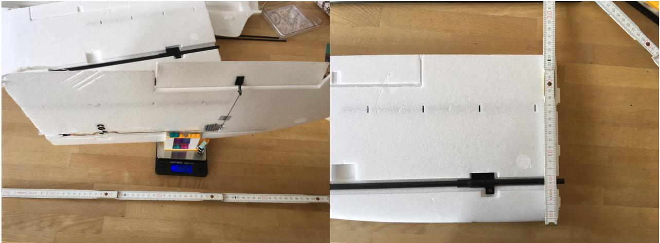
Figure 8: Right wing with servo and beam 140.5g
