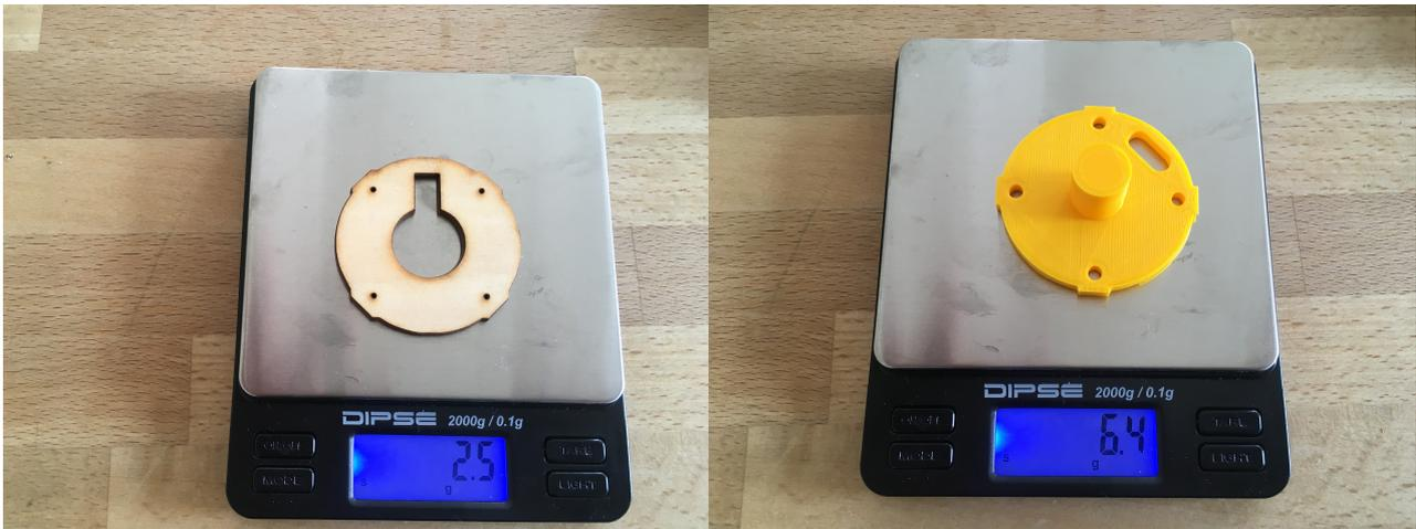
Figure 6: Motor mount. Left: Original wood version (2.5g). Right: 3D print version (6.4g)
