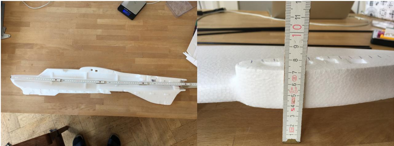
Figure 3: Fuselage length 810mm excluding motor and width 70mm
