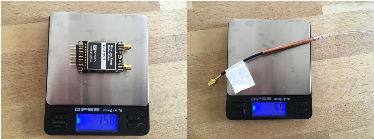
Figure 18: RFD868+ modem (15.8g) and antenna (6.7g)
