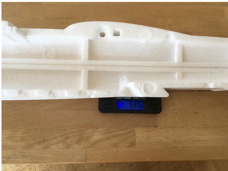
Figure 1: Fuselage half foam only - 58.5g
