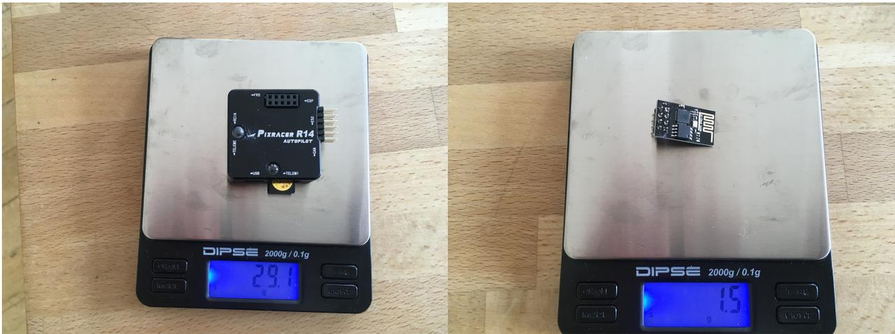
Figure 16: Left: PixRacer with Alu case and memory card (29.1g). Right: Wifi module (1.5g)
