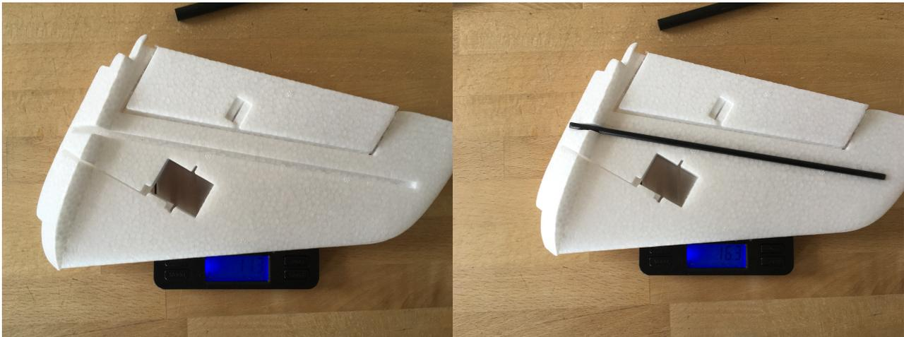
Figure 12: Vtail wing without beam (11.3g) and with beam (16.3g)
