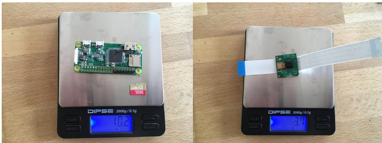
Figure 23: Left: Raspberry Pi Zero W (10.2g), Right: Raspberry Camera (3.7g)
