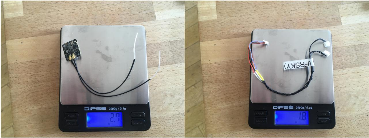
Figure 17: FrSky RC receiver (2.7g) with cable (1.8g)
