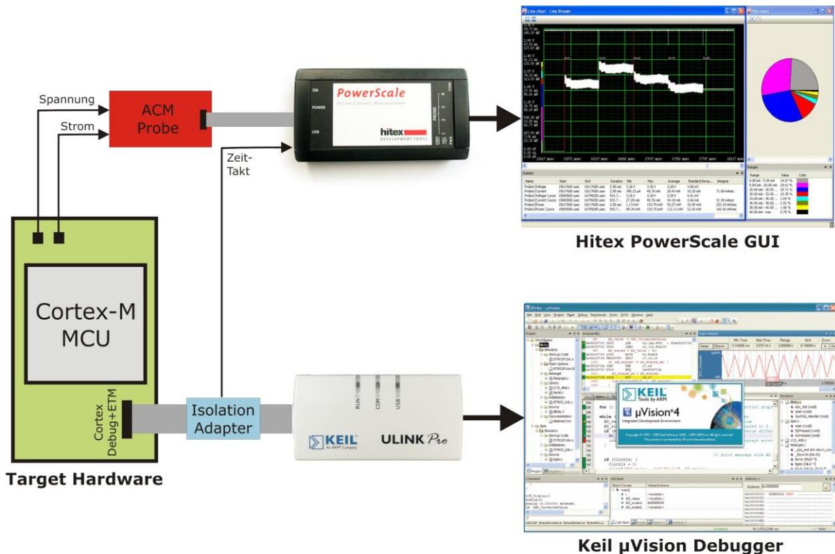
Figure 8: PowerScale and ULINKpro connected to the microcontroller system.
