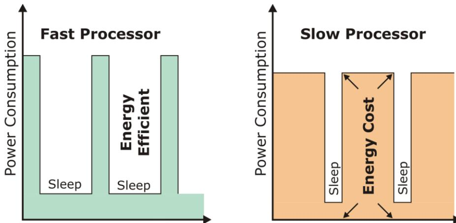
Figure 1: A faster microcontroller needs less processing time for algorithms, is therefore longer in power-saving modes and can be more energy efficient.
