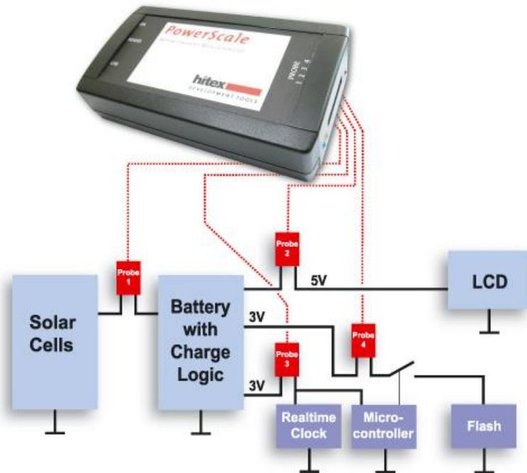
*Figure7: PowerScale measures the current and voltage on up to four power domains.*
