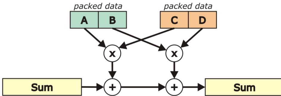
Figure 6: SIMD extensions perform multiple operations in one single-cycle CPU instruction, in this example:  $Sum = Sum + (A \times C) + (B \times D)$
