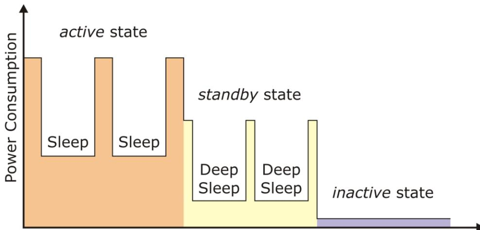
Figure 2: power profile of a microcontroller application
