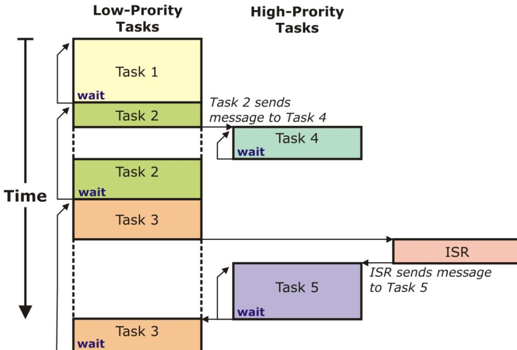
Figure 3: task and interrupt execution of an RTOS system
