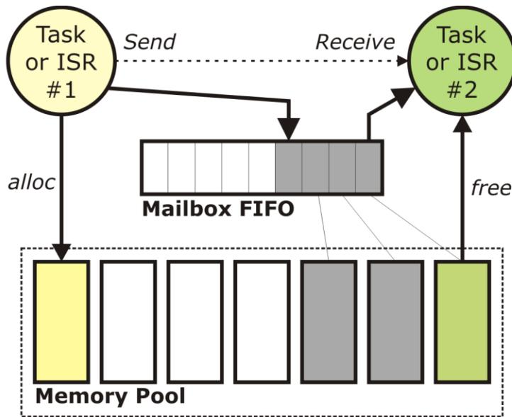
Figure 4: Block I/O operations in RTOS use memory pools and a mailbox FIFO for communication
